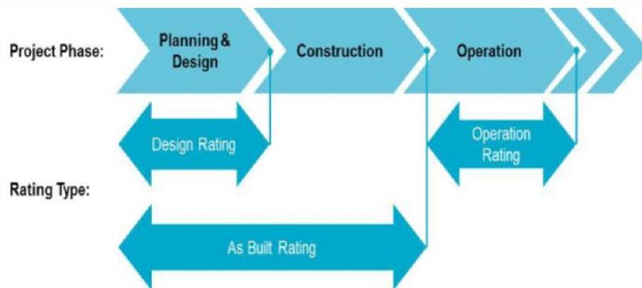
Fig 3. Different modes of IS rating tool and project phases
